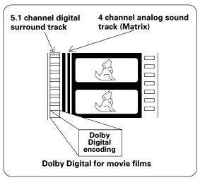
The number of movies made using Dolby Digital since 1992 has exceeded 300 and continues to increase. For compact disc players and laser disc digital sounds, 16 bits are used to sample the original analog audio waveform and sampling is carried out 44,100 times every second. However because an enormous amount of recording signal data is required for the multi channel system with this method, Dolby Digital is used to compress the data.
